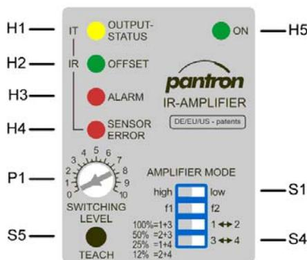
**H1:** Output status indicator - yellow, illuminated when the switching output is active
